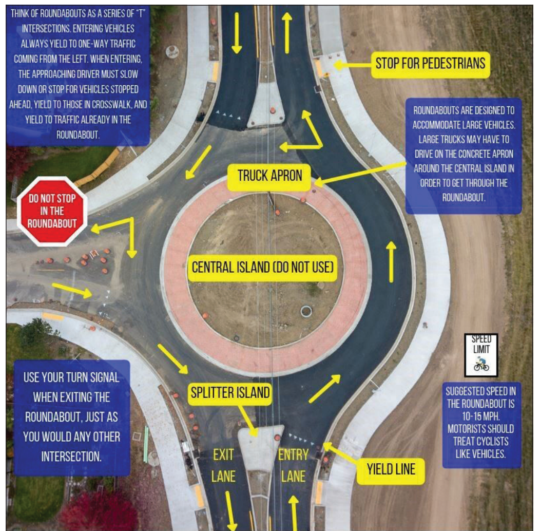
Roundabouts permit traffic to flow efficiently in one direction by allowing drivers to follow a gentle curve.
